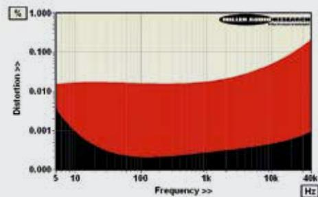
**ABOVE:** THD vs. extended freq for N°523 preamp (1V out, black trace) vs. N°534 amplifier (10W/8ohm, red)
