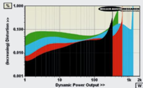
**ABOVE:** Dynamic power output versus distortion into 8ohm (black trace), 4ohm (red), 2ohm (blue) and 1ohm (green) speaker loads. Max. current is 25.0A
