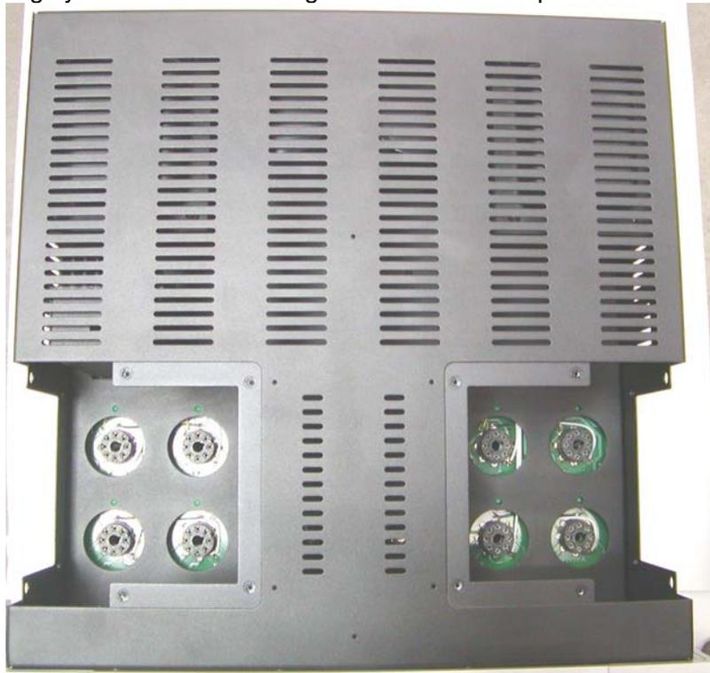
5. Insert the output tubes into each of the output tube sockets from tube # 1 to # 4 on the left side of the cover and 5 to 8 on the right side of the cover.
