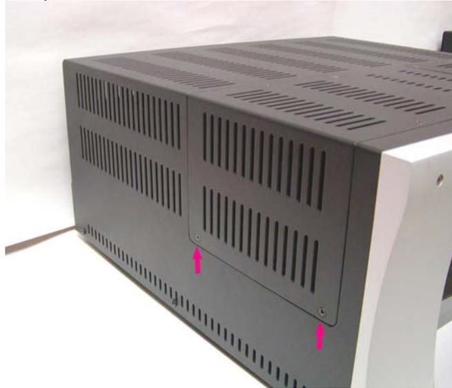
3. Save these screws in a safe place so that they can be re-used to fasten the cage back to the amplifier.
