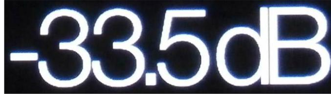
When the **Balance** menu page is open or the remote **Balance** button has been pressed, the rotary control adjusts the channel **Balance** instead. The Balance adjustment is in 0.1dB steps down to -6.0dB on each channel, then mute ( $-\infty$ ) below that. The **Volume** taper on the display changes to show the **Balance** setting.
