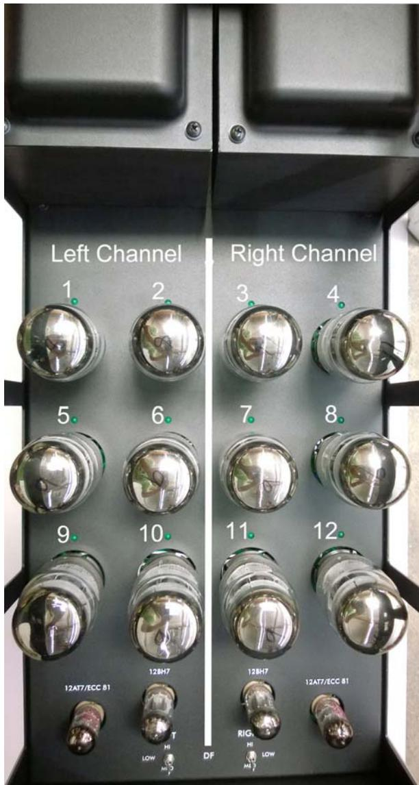
1. Plugging in a new tube: Hold onto the upper portion of the tube towards its tip. Lower the tube onto the socket, making sure that the pins from the tube match the holes in the socket.
