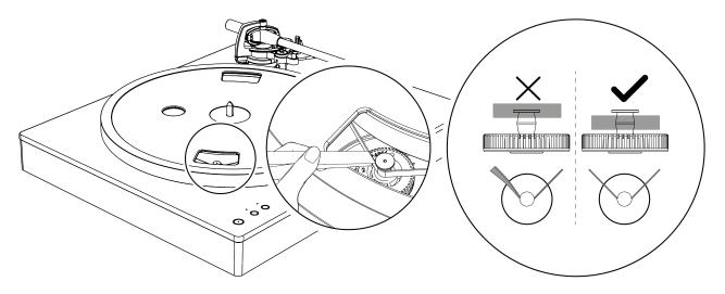
3. Push and rotate counterweight onto tonearm and then carefully insert the headshell into the tonearm.
